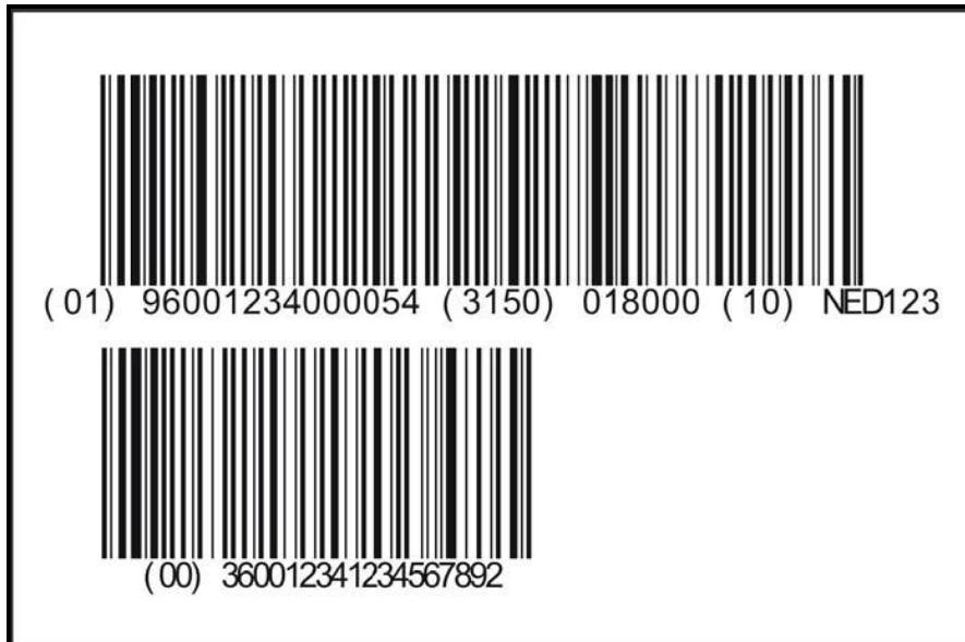
The SSCC and attribute information bar coded in a GS1-128 symbol
